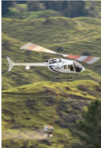
2,000 lbs. Cargo Hook Capacity and Cargo Weighing System
